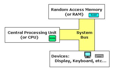
The **system bus** (shown in yellow) connects the various components of a computer.
